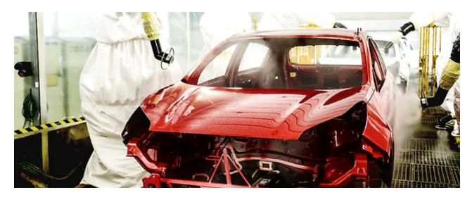
Paint Spray Booth is an enclosed area where car body painting is processed. In this unit, there is a water circulation on the wall catching up the over spray paint. The mixture of over spray paint and water should be treated if do not want to have any problem such as formed clumps of sticky paint, blockage of mist eliminator, shower head and circulation pump.
